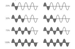
Cycle Control method is a method of making a loaded power as proportionally repeated ON/OFF cycle by a signal of input control in a fixed cycle. The proportionally repeated ON/OFF cycle makes the power applied to the load be regularly. This method is better than Phase Control since this control method makes the loaded power be ON/OFF at the zero point of AC when it is ON/OFF so that there is almost no noise occurrence and it is better for the linearity compared to the Phase Control.
